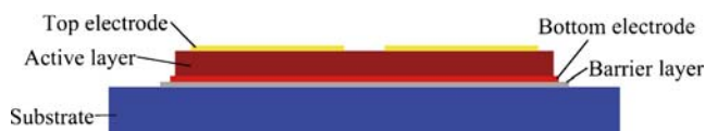
Fig. 1 A cross-sectional view of the entire structure. The barrier layer is only necessary when a silicon substrate is used
