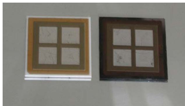
Fig. 2 A picture of the actual structure taken with a digital camera. Alumina substrate on the left and silicon substrate on the right . Each sample is 30×30 mm 2
